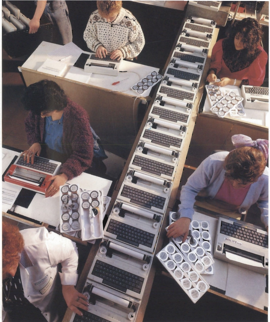
Britains Petite workers in Nottingham, England, are busiest before the holiday season, inserting HP's ink-jet cartridges into lightweight electronic typewriters.
